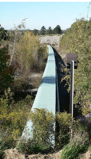
A covered conveyor takes gravel from the source in an Niagra Escarpment open pit aggregate mining operation. PHOTO COURTESY SIGHTHOUND/FLICKR
