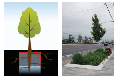
Tree cell schematic (left). Underground tree cells, in York Region (right)
